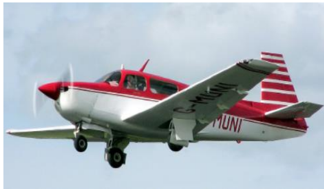
Figure 1: Tricycle landing gear
